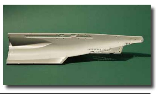
The deck ports are a different class. The remaining material is only 1/2 mm and therefore very brittle. On the other hand the ports are so small that they will be blocked by a thin film of water immediately.
