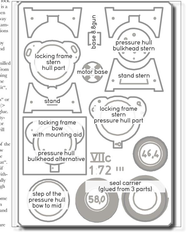
kind of bayonet lock. The seal carrier is a loose ring between the parts. This way the full access diameter to both sections stays open. The locking is done by 3 screw heads and keyholes.
