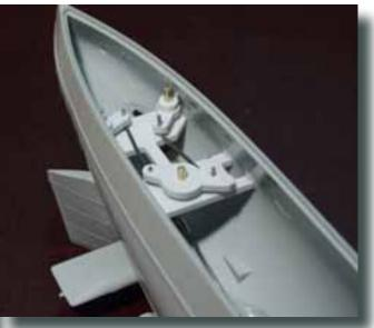
plate can be found in the 2mm cut plate. The rudder shafts are 2mm brass and the linkages ø 1 mm St/St. The corresponding holes have to be bored following the markings on the parts.
