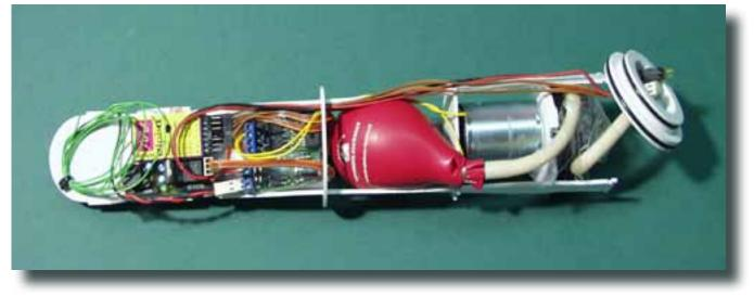
cated quick-divers. Taking this into account the biggest possible pump is installed into the model. It is tricky to mount, but will let the model dive within 30 sec.
